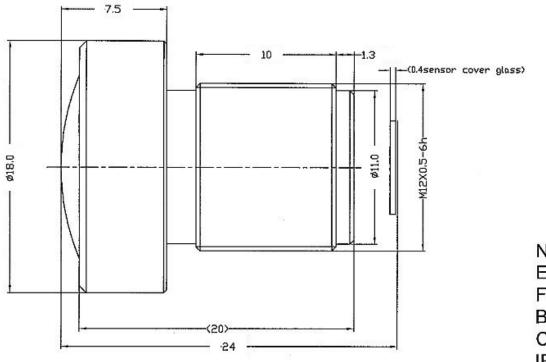
Notes: EFL=2.33 F#=2.8 Barrel material: AL Cap material: AL IR cut coating: T=50%@670±10nm
